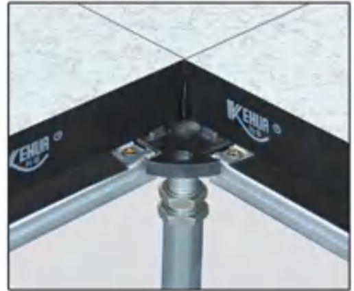
Positioning point function (to prevent floor deviation)
